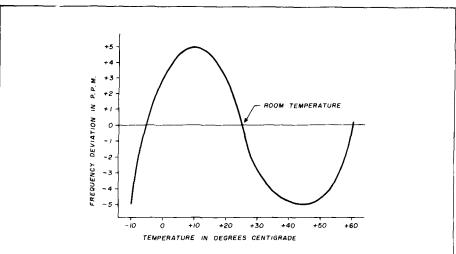
fig. 4. Typical frequency drift versus temperature for an "AT" cut high-accuracy crystal at 4.000 MHz.
